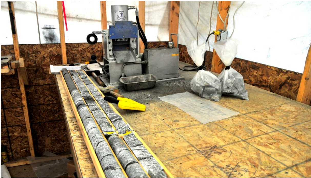
Figure 11.4 - Hydraulic Core Splitter in the Core Shack
