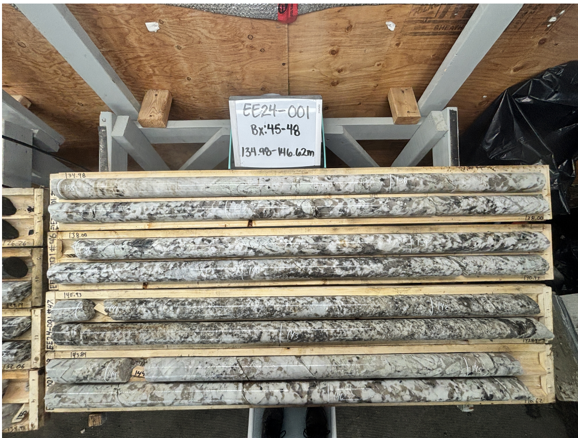
Drillhole EE24-001, core samples from 134.98 m to 146.62 m, visually estimated spodumene of 14%.
